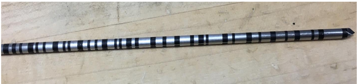
Figure 15 - The wire address scheme is shown here. Addresses are separated by a 2.5mm thick line.
